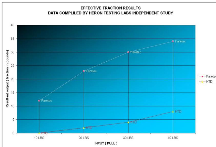
Interestingly, while 4:1 traction is the theoretical mechanical advantage, the experimental traction provided is still less than 1:1. For 40 pounds of force, the output traction is less than 35 pounds. And for the KTD the output is less than 10 pounds. Never underestimate friction!
